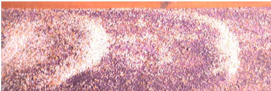
Figure 3.18: Sample photographs for deposition of sediment at lee face.
